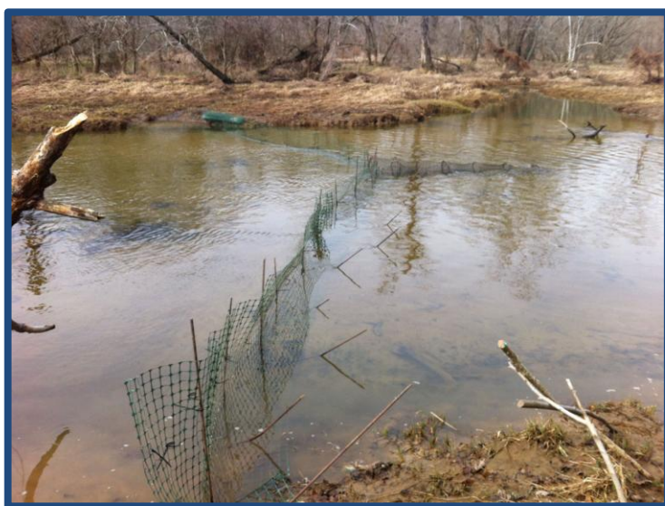
Figure 1. Hoop net deployed in Pohick creek. The top of the hoop net is exposed at both high and low tide to avoid drowning turtles, otters, or other air-breathing vertebrates. The hedging is angled downstream in order to funnel up-migrating herring into the opening of the net.
