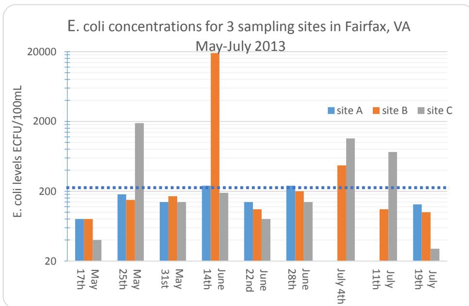
Figure 1: Bar graph of the three sampling sites by date to show the differences in *E. coli* concentrations. The sites are color coded and the blue horizontal line represents the 235 CFU/100mL standard for recreational waters.
