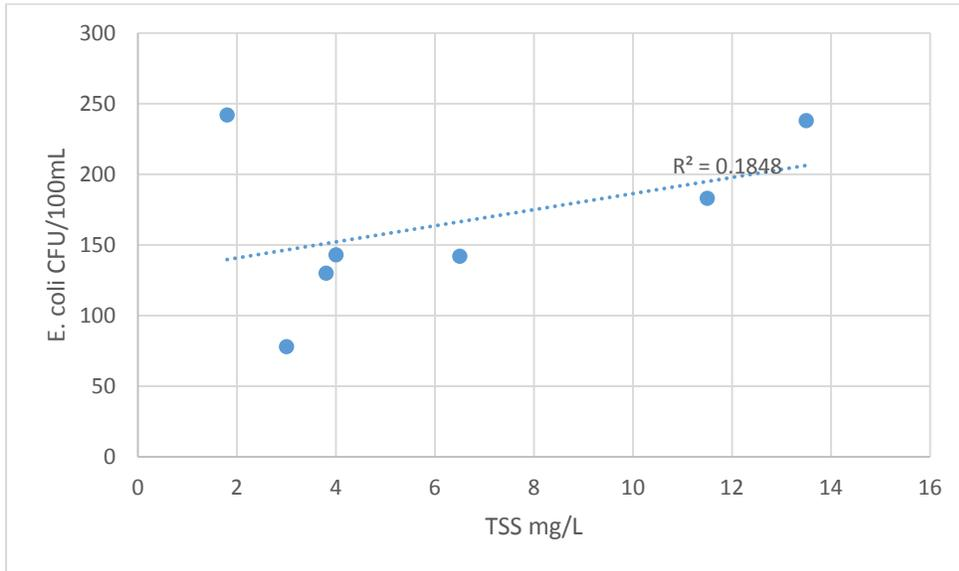
Figure 2: Site A- *E. coli* (CFU/100mL) vs TSS (mg/L), n=7 (two samples were noted as tmtc and excluded from the analysis)
