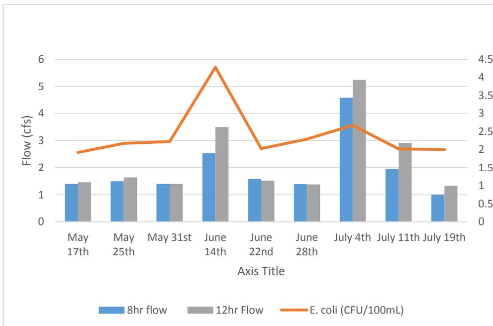
Figure 5: Relationship between flow and *E. coli* log<sub>10</sub> concentrations at Site B on the 9 sample days. Blue bars represent the 8 hr average flow (ft<sup>3</sup>/s), the grey bars represent 12 hr average flow, and the orange line represents the *E. coli* levels (CFU/100mL).
